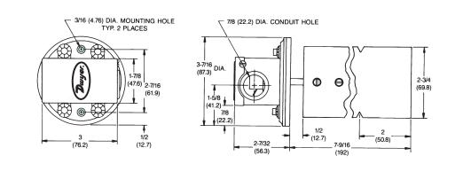
**The Model 530 Air Flow Switch** provides excellent sensitivity and reliability at a very reasonable price. Quality features include rugged die cast zinc body, stainless steel vane, silicone rubber gasket and SPDT snap switch. Unit is easily field adjustable from 400-1600 FPM. Mounting is fast and simple, requiring only two screws. Vane fits 6 in. or larger ducts. UL approved. To order, specify Dwyer Instruments, Inc. Model 530 Air Flow Switch.
