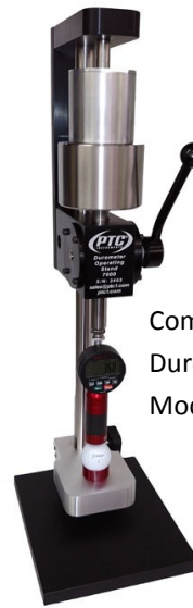
Compatible Deadweight Durometer Test Stand Model 479
