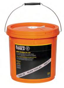
The Klein Tools 1250-Pound tensile strength conduit measuring pull tape is a durable, flat polyester strapping that disperses pull load and minimizes stretching when pulling. The tape is marked with descending 1-Foot increments to measure conduit runs. Tape is pre-lubricated to reduce friction and comes in a bucket with a hole in the lid for tangle-free dispensing. Pull Tape is also available in a variety of tensile strengths and lengths.
