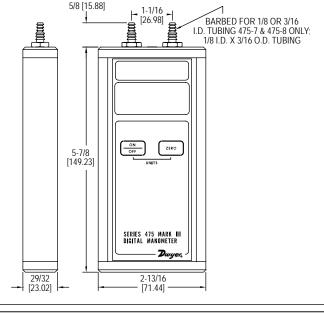
The Series 475 Intrinsically Safe Handheld Digital Manometer measures positive, negative, or differential pressures of air and natural gases in ranges from 1 in w.c. (0.249 kPa) to 150 psid (10.34 bar). The dual push pads on the front panel control the on/off, auto zero, and pressure unit selection, allowing for simple operation with no set up needed. When used with a Dwyer® Pitot tube (①), the Series 475 can also be used as an air velocity gage.
