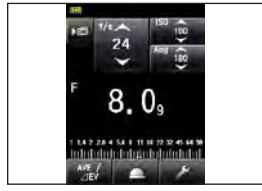
The L-858D offers frame rate, shutter angle, illuminance (lx, cd/m2) and luminance (fc, fl).
