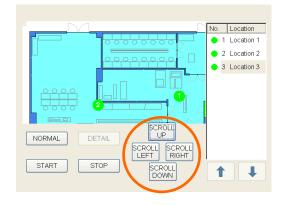
When a MAP is enlarged, [SCROLL UP], [SCROLL DOWN], [SCROLL LEFT] and [SCROLL RIGHT] buttons are activated, which enables you to move the MAP.
