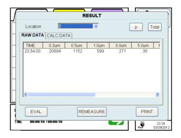
When all measurements are finished, the final measurement results will be displayed. You can view the result of a certain LOCATION POINT by selecting Location from the dropdown list.
