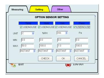
In the OPTION SENSOR SETTING screen you can confirm if the option sensor is connected or not, and whether or not to use the sensor.
