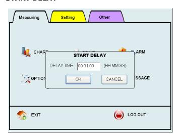
In the START DELAY window set a measurement delay time.
