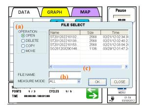
(a) To display names of every saved file, check "OPEN". (When this screen is open, "OPEN" is selected by default.)
