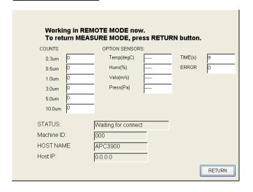
Change to REMOTE MODE to perform a measurement from a PC connected via Ethernet using the remote sampling software.
