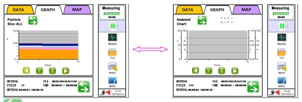
: Switches the display between the particle chart and the OP sensor chart on the GRAPH screen.
