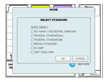
Tap [STANDARD] to open the SELECT STANDARD window to select a measurement standard to be applied in the STANDARD mode.
