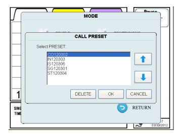
Select the item that you want to load or delete. Tap [OK] to load the selected PRESET settings into MODE and MEASURE SETTING (Authentication required).
