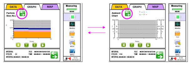
Scrolls the chart to the left (half of the display can be scrolled at a time).
