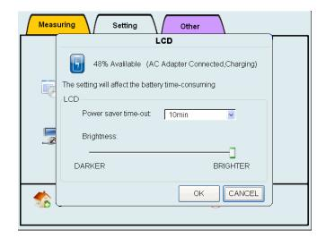
In the LCD settings, configure the Power saver time-out and Brightness setting. Also the LCD displays the power state of the unit (battery level, power source (AC/battery), battery charging, etc.).
