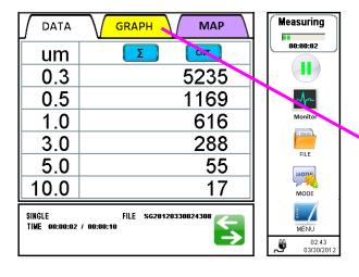
Tap GRAPH to switch to displaying a chart while measuring.
