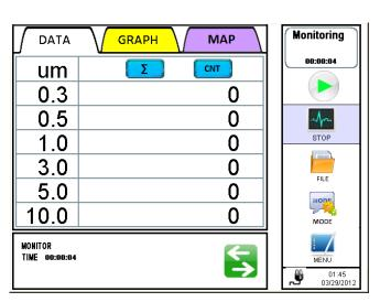
Tap [MONITOR] on the initial screen to start monitoring. Sampling will start in 10 seconds after the pump starts operating.
