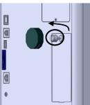
Open the battery compartment cover on the rear of the instrument.
