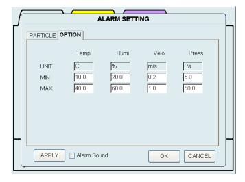
In ALARM SETTING you can set thresholds for the particle alarm and option sensor alarm.
