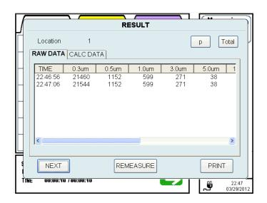
When a measurement is finished, a measurement result window will be displayed.
