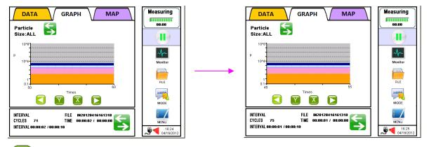
Scrolls the chart to the right (half of the display can be scrolled at a time).
