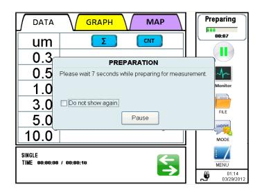
Tap [START] on the main screen to start a measurement using the settings configured in **3.5 MODE** .
