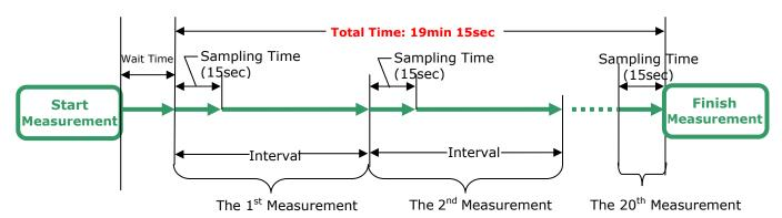
If the time period between two samplings is 10 seconds or longer, the pump will be turned OFF after a sampling is finished. Then the pump will be turned ON again 10 seconds before the next sampling starts.
