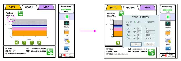
Select either LOG or LINEAR for the Y axis. Select the maximum scale value from four options. For setting the four maximum values, please refer to 3.8.1 MEASURING – CHART SETTING. In the display shown above, LOG is selected for the scale of the Y axis and the maximum scale value of the Y axis is set to 10 to the sixth.
