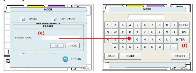
Tap [PRESET] (d) on "MEASURE SETTING" dialog box to display a window asking you to input PRESET NAME.
