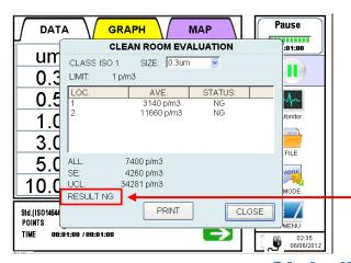
When a measurement at each location is finished, the measurement results will be displayed.
