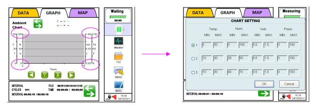
Select one of the three combinations of minimum and maximum scale values of the Y axis for each sensor. For setting the combination of minimum and maximum values, please refer to 3.8.1 MEASURING – CHART SETTING.
