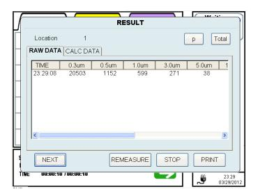
When a measurement at each location is finished, the measurement results will be displayed.
