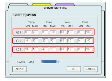
In the OPTION tab, configure the "MIN" and "MAX" settings for each sensor.
