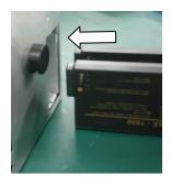
When you plug in the AC adapter, the Power state LED will light up red. When the batteries are charging, the red LED will blink.
