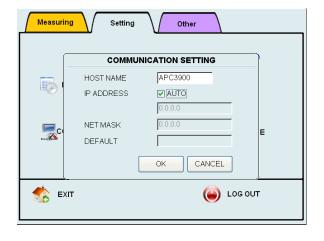
In the COMMUNICATION SETTING, configure the settings for Ethernet connection. This settings need to be configured when connecting the instrument to a PC using remote console or remote mode.
