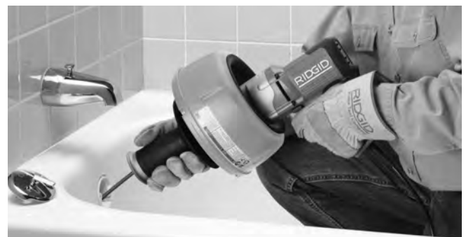
Figure 9 – Push Cable Down Drain Line
