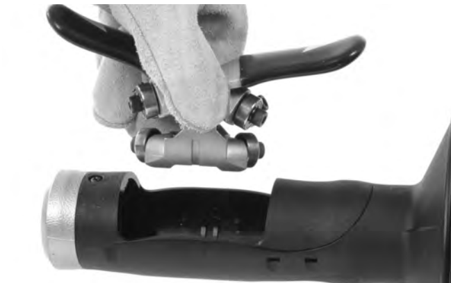
Figure 12B – Removing AUTOFEED Mechanism From Housing
