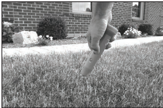
HotWire Hound locates boundary wire using null method.
