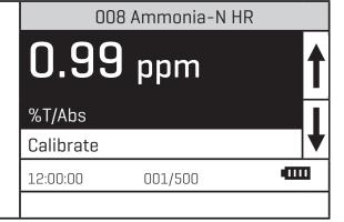
11. Press enter to select **Calibrate**. A reverse font (light background with dark characters) will appear to indicate that the reading can be adjusted.
