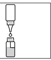
7. Use 1.0 mL pipet (0354) to add 1.0 mL of \*Ammonia Nitrogen Reagent #2 (V-4798).
