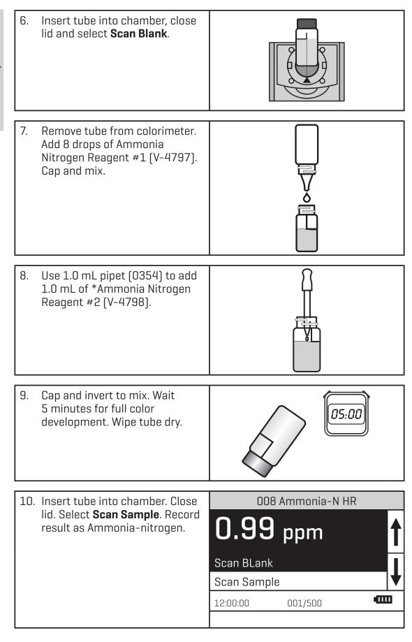
NOTE: The meter will remember the last scanned blank reading. It is not necessary to scan a blank each time the test is performed. To use the previous blank reading, instead of scanning a new one, scroll to Scan Sample and proceed. For the most accurate results, the meter should be blanked
