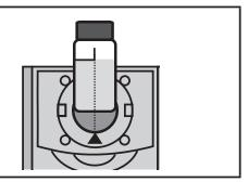
6. Remove tube from colorimeter. Add 8 drops of Ammonia Nitrogen Reagent #1 (V-4797). Cap and mix.
