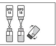
8. Immediately insert tube into chamber. Close lid. Select **Scan Sample**. Record result as Free Chlorine.
