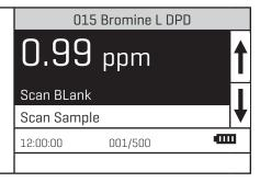
NOTE: For the most accurate results, samples over 7 ppm bromine should be diluted with chlorine demand free water and re-tested.
