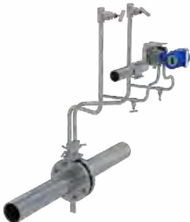
For liquid flow measurement, up-tilt the guiding pressure tube by 45°. Ensure that transmitter installation location is at lower level than that of the process pipeline. Pre-inject cooling liquid into the guiding pressure tube. Slowly open the shut-off valve to start measurement. Periodically open the drain vent to clear the residual gas from the guiding pressure tube, which will improve the measurement accuracy.
