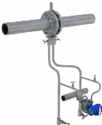
For liquid flow measurement, tilt down the guiding pressure tube by 45°. Ensure that transmitter installation location is at lower level than that of the process pipeline. Pre-inject cooling liquid into the guiding pressure tube. Slowly open the shut-off valve to start measurement. Periodically open the drain vent to clear the residual liquid, which will improve the measurement accuracy.
