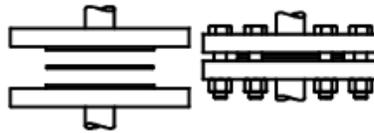
Choose gasket according to the properties of the process medium and the temperature range. Pay attention to the bolt balance lock
