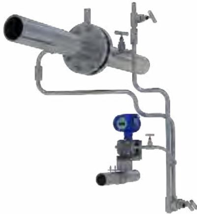
For steam flow measurement, up-tilt the guiding pressure tube by 45°. Ensure that transmitter installation location is at lower level than that of the process pipeline. Pre-inject cooling liquid into the guiding pressure tube. Slowly open the shut-off valve to start measurement. Periodically open the drain vent to clear the residual steam from guided pipeline to improve the measurement accuracy.
