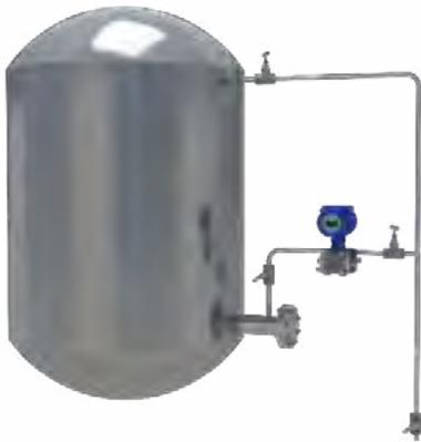
Use a single flange diaphragm system for sealed container level measurement. Increase the isolation tank and multiple shut-off valves. Periodically open the drain/vent valve to clear off the residual gas and liquid in the guiding pressure tube for higher accuracy.
