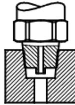
Use tapered thread connections to make better seals. Sealing with Teflon tape or sealant glue results in strong and leak resistant connections.
