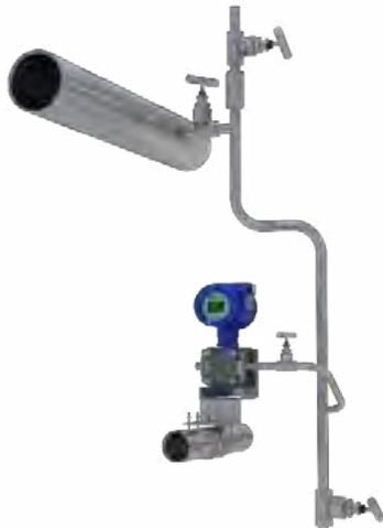
For high temperature steam measurement in a pipeline by differential pressure transmitter, pre-inject cooling water into the guided pipe. Once the steam pipes are stable, slowly open the shut-off valve and start measuring.
