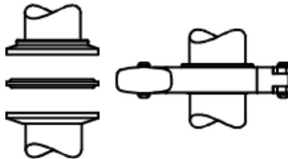
Choose gaskets that meet specified standards to avoid excessive clamp locking and squeezing gasket. Excessive locking of clamp may damage the sensing diaphragm and cause measuring error.
