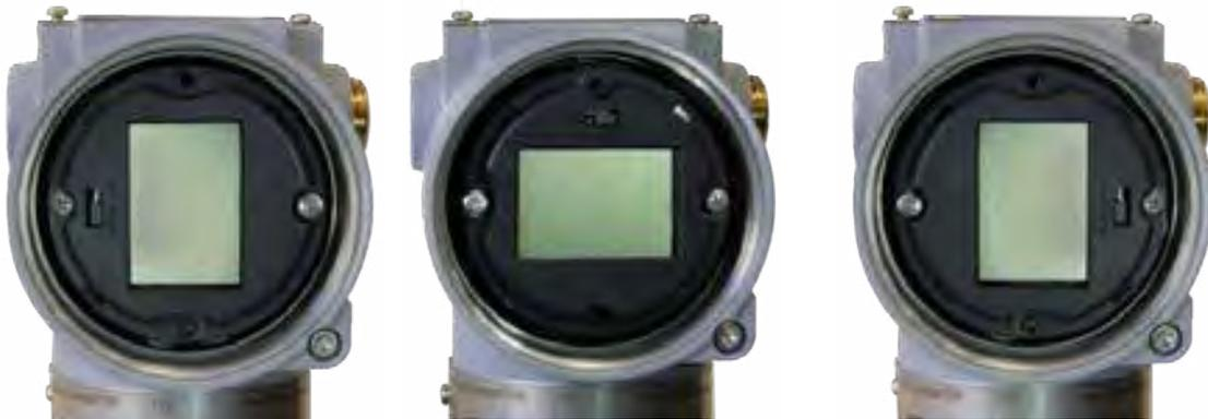
The alignment of the display device can be adjusted vertically or horizontally as per the requirement of installation location. Unscrew the screws on either sides of the LCD screen to rotate it 90° clockwise or counter clockwise. The figure below illustrates the vertical and horizontal arrangement of the display device.
