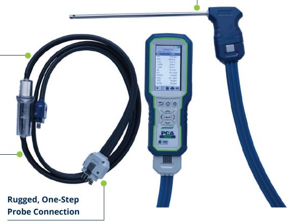
Provides a quick, simple, durable connection to the analyzer.
