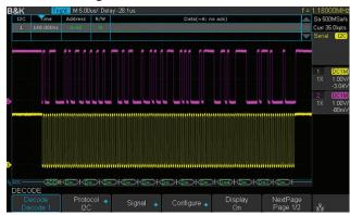
Serial bus decoding supports I<sup>2</sup>C, SPI, UART, CAN and LIN protocols. Information can be quickly displayed in a tabular format.
