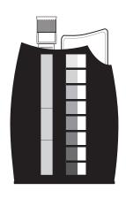
The Octa-Slide 2 Viewer should be held so non-direct light enters through the back of the Viewer. Insert the Octa-Slide 2 Bar into the Viewer. Insert the reacted sample into the top of the Viewer. Match the color of the reaction to the color standards.
