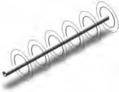
Figure 1 – The field emitted by a charged line.
