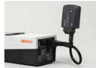
Example of the connection with SJ-210
