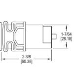
The Series TID Temperature/Process Indicator displays temperature or a process value measured by a PTC or NTC thermistor or a 4-20 mA transmitter.
