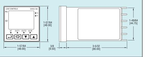
Monitor and control temperature or process applications with precision using the Series 16B controllers. The units offer two separate outputs for dual loop control in direct or reverse acting. Select relay, voltage, or current output combined with a second relay output.
