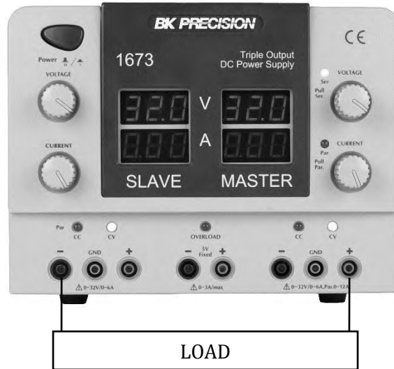
Figure 5 – Series Tracking Mode Load Connection
