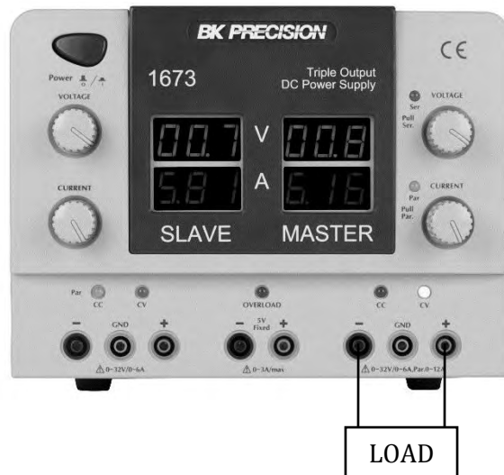
Figure 6 – Parallel Tracking Mode Load Connection
