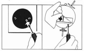
Line up the adjustable needle with the barometer needle daily.
