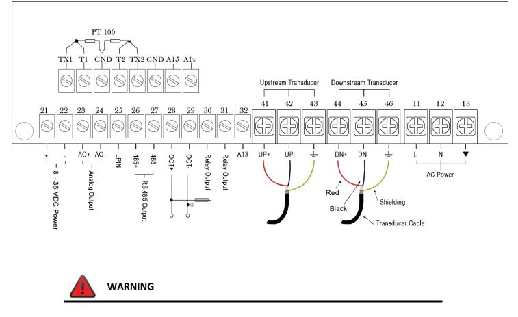
• Make sure to connect to ground the power board terminal block
