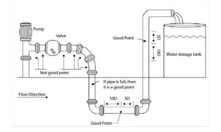
The above figure shows the installation point of transducers when a compressor is used in the pipeline.
