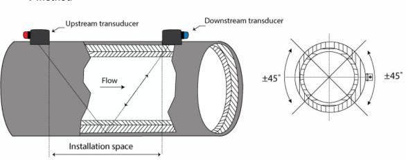
V method is a standard installation method and convenient to use for precise measurement of flow. While installing the two transducers, they're horizontally aligned. They are suitable for pipe diameter range  $\frac{1}{2}$ " to 16" (DN15 mm-DN400 mm).
