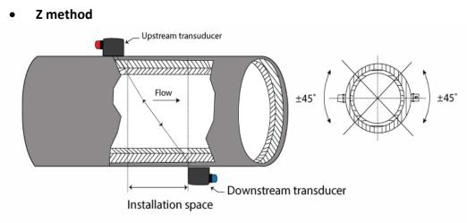
When the pipe diameter is wide, or there are suspended matters in the fluid, or the scaling is too thick and interferes with the normal functioning of the flowmeter and weakens the signal in a V method installation, then Z method installation is used. It is also called the single sound path as it can directly transfer the pulse without any reflection required as is required in case of V method and therefore has less signal attenuation.
