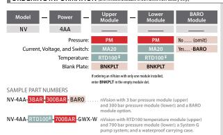
‡ RTD100 does not include a temperature probe. Please choose a probe from the list below, or from a more comprehensive list on our website under Accessories. Alternatively, connect to your own probes with the supplied RTD100 mating connector.
