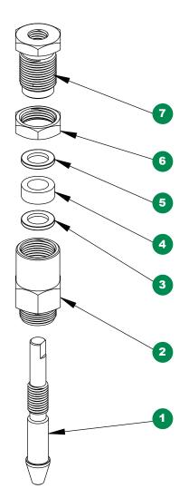
1 Mini valve packing stem 2 Mini valve packing bonnet 3 Packing washer
