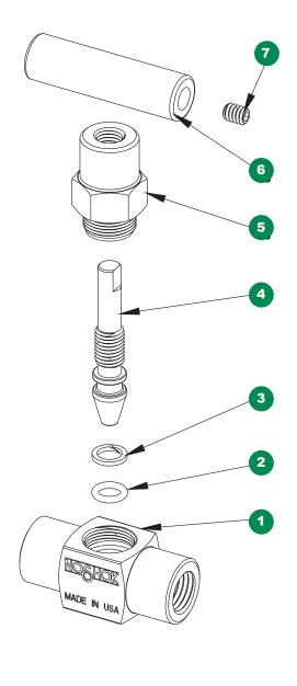
1 Mini valve body 2 FKM o-ring 3 PTFE back-up ring 4 Mini valve stem 5 Mini valve bonnet 6 Mini valve "T" handle 7 Set screw
