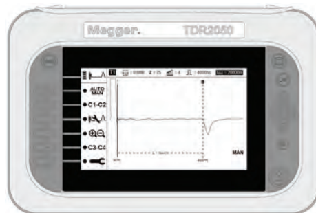
Figure 3 – Trace of a Short – Negative Reflection – Conductors Moving Closer Together
