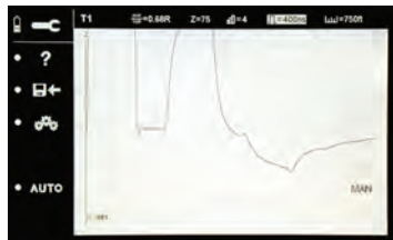
Figure 5 - Pulse Width and Dead Zone
