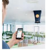
Bluetooth App allows for hands free operation, displaying measurement data on mobile devices and finalizing and sending the measurement report via email from the job
