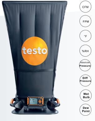
The new testo 420 flow hood system is light, accurate and a convenient solution for balancing volume flow at supplies and returns. At turbulent outlets, the flow straightener significantly improves measurement accuracy, saves time and eliminates the uncertainty of measuring turbulent outlet ducts. Handling is especially easy with its ergonomic handles and low weight of less than 6.4 lbs. The 420 Differential Pressure instrument can be tilted for optimum viewing angle.
