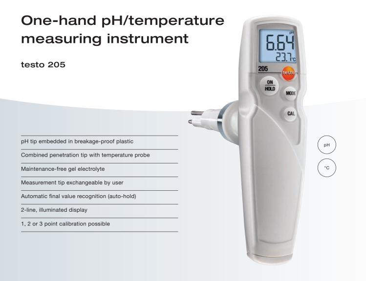
The testo 205 is a robust food penetration measuring instrument for temperature and pH values, with automatic temperature compensation. The robust penetration measurement tip is exchangeable and insenstitive to dirt thanks to the hole diaphragm.
