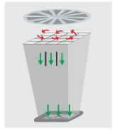
Functional principle of the flow straightener.
